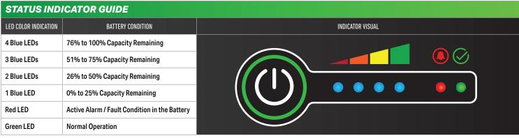
The Trojan® GC2 36V Lithium-Ion features include a battery status push button and indicator light on the top of the case. A momentary press of the button displays the battery's State of Charge and operating status.
